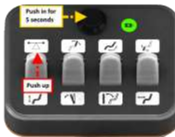
Figure 8-1: System Homing – Switch Positions
